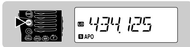
**Note:** Selecting lower transmit power is a wise method to reduce battery consumption if communication is still reliable.
